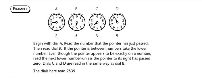
**Directions** Record the readings on these sample utility meters.
